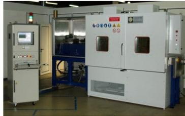
SDI's pulsed air test systems are designed for the global equipment suppliers or car manufacturer involved in the use or production of air ducts and pipes. Our solutions allow prototyping, characterization and durability testing to ensure quality and compliance with automotive and aeronautic industries standards
